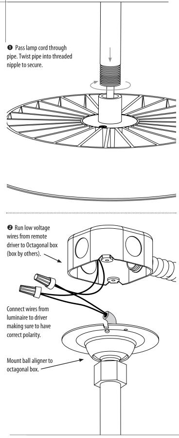
Drivers must remain accessible after finished installation. Driver housings must not be mounted closer than 4 inches apart. Maximum distance from lamp to driver is 100 feet, with 10AWG wire.
